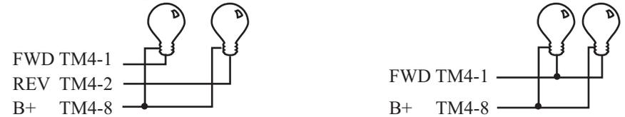
**1.5 Volt Bulbs:** Miniature, 1.5 volt bulbs must use a series limit resistor. A single limit resistor may be used as shown. This assumes that only one lamp is on at a time. Lower resistance values will increase the lamp brightness but shorten the life of the bulb. For best results, use the highest resistance compatible with bulb visibility. Always know the ratings of the bulb to be used.
