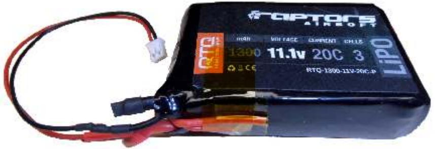
Finished LiPo battery pack with charging connector and power connector removed. Unused wires have been shortened. The power output wires are covered by heatshrink tubing. The two unused charging wires were covered the orange Kapton tape and stuck to the bottom of the battery.
