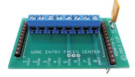
Parts are inserted from the top side and soldering is done on the back or bottom side of the circuit board.
