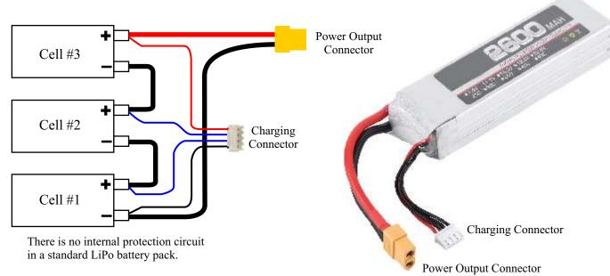
Which LiPo connector is used for AirWire? If you have the space, get a matching connector and use the power output connector. The disadvantage of this approach is the space taken up by the bulky wire and connector.
