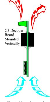
Vertical board mounting allows better airflow
