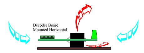
Mounting the decoder horizontally is OK but the airflow is blocked by the board itself
