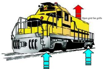
**Airflow In Modern Plastic Diesel Locomotives**
