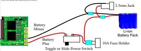
**Do Not Use The Locomotive's Internal Circuit Boards -** Do not attempt to use any of the loco's built-in circuit boards for wiring and connections especially to the motor. This is one of the most common causes of decoder damage and or failure of the constant speed feature.
