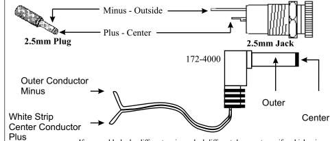
If your cable looks different or is marked different, be sure to verify which wire connects to which part of the plug. Incorrect polarity applied to the G3 will damage it.
