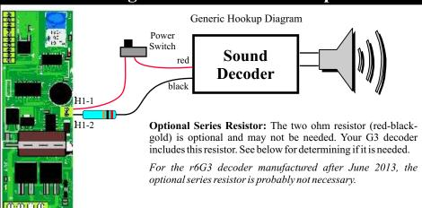
**DCC Sound and Multi-Function Decoders:** Before using a DCC sound or multifunction decoder, check the manual or call the manufacturer to verify that it will withstand the battery voltage you will be using. Some older sound decoders, such as the Soundtraxx DSX are rated only up to 18 volts.
