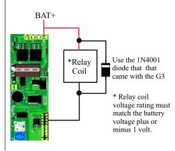
A relay or a solenoid can be driven by the G3 LED drivers. Just be sure that their rating matches your battery voltage.
