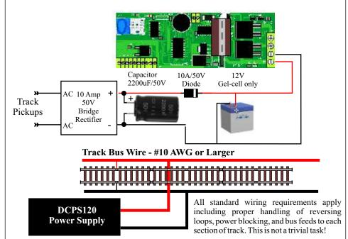
The DCPS120 Power supply is a 120 Watt, adjustable DC power supply with excellent load regulation. The output voltage is variable from 15V to 24V. It has built in overload and short circuit protection. It is available direct from CVP Products. See the website for ordering details.
