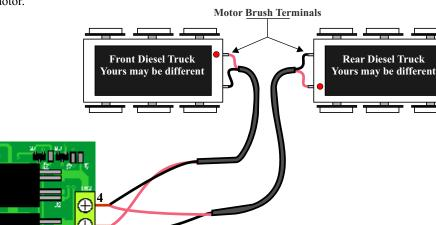
Use a stiff piece of copper wire as a connection point for the two motor wires. This is easier than twisting two large wires together - the twisted and tinned wires may not fit the terminal. Do not allow the wires to touch any metal objects. Do not allow the motor wires to short together.
