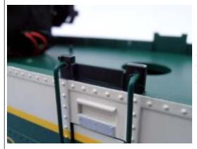
The side doors and handrails are part of the top chassis and do not have to be removed. They don't connect to the bottom chassis.
