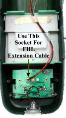
After unplugging the red/white plug from the nose circuit board, plug it into the CAB header on the Drop-In. This provides for independent control of the cab interior lighting.
