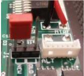
Warning - If you set the jumper for OLD, and your locomotive actually is a newer model that uses low voltage bulbs, you will burn out every bulb in the locomotive. If unsure leave the jumper set for NEW.
