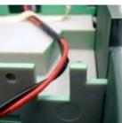
Plug in the extension cable to the left most socket on the cab's circuit board. This insures the correct lights will be on when the loco is moving forward. The other two sockets are unused.
