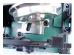
**Enlarge Switch Opening In Chassis Floor**
