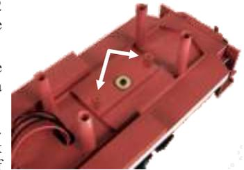
The battery is mounted to the chassis using double-sided tape. Build up several layers to insure the battery clears the truck mounting screw. See the note below about the desired type of tape to use.
