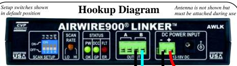
All Activators share the same two wires that come from a single Linker. However, there may be more than one Linker and each Linker will have its own Main Bus. Individual Linkers can not be paralleled nor can they share a Main Bus.
