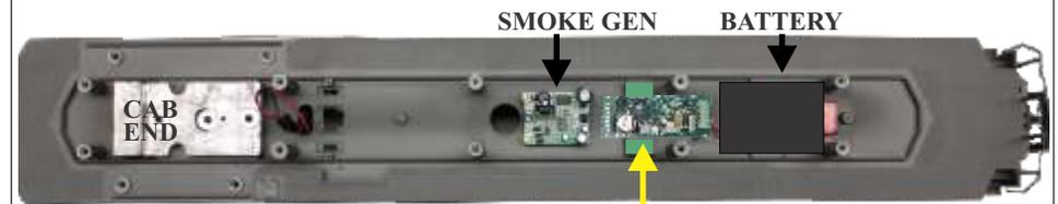
It is best to attach a thin piece of plastic to bridge across the two cast-in boxes where the sound decoder will be mounted. The sound decoder mounts to the bridge. Use a piece of thin styrene or other similar material. VHB tape attaches the bridge to the boxes.
