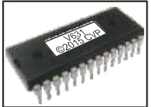
Socketed software chip for easy upgrades
