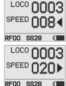
The top image to the right shows loco 3 is set for speed step 8 and for the reverse direction.
