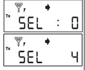
Push any number from 0 to 7. For this example, frequency 4 will be selected. To enter the new frequency, push #. The change takes effect immediately.
