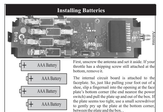
The battery orientation is marked on the circuit board. Note the batteries all face the same direction with the plus end towards the bottom, away from the antenna.
