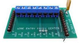
Parts are inserted from the top side (side with white lettering) and soldering is done on the back or bottom side of the circuit board.
